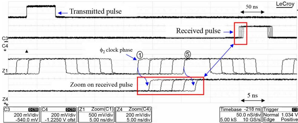
Fig. 3. Latency between transmitted and received pulse for different clock skews.
