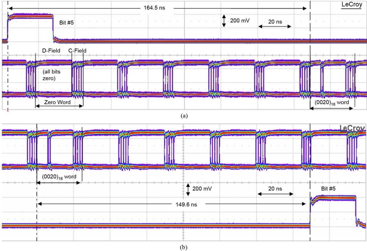
Fig. 11. Oscilloscope screen-shots showing the latencies of the transmitter and of the receiver. (a) Upper trace: transmitted payload bit. Lower Trace: CIMT encoded serial stream. (b) Upper trace: CIMT encoded serial stream. Lower Trace: received payload bit.
