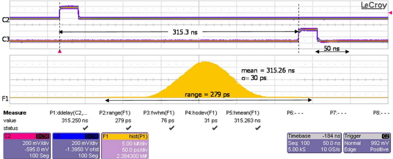
Fig. 10. Histogram of the latency of the link. Topmost trace: transmitted payload bit. Second trace: corresponding received bit. Down: histogram of the latency.
