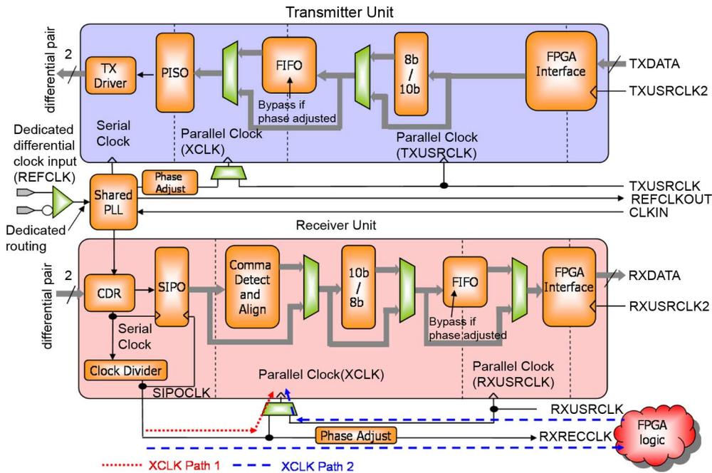
Fig. 4. Simplified block diagram of Xilinx GTP transceivers. Half a tile is shown.
