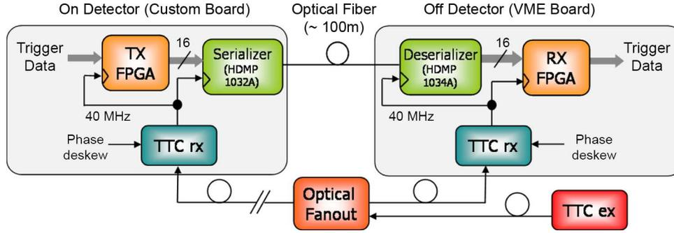
Fig. 1. Simplified block diagram of the serial link setup in L1 ATLAS barrel muon trigger.
