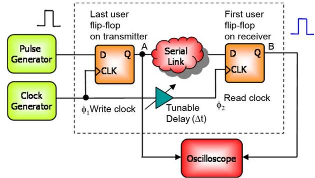
Fig. 2. Synchronous serial link with skew on clock distribution.
