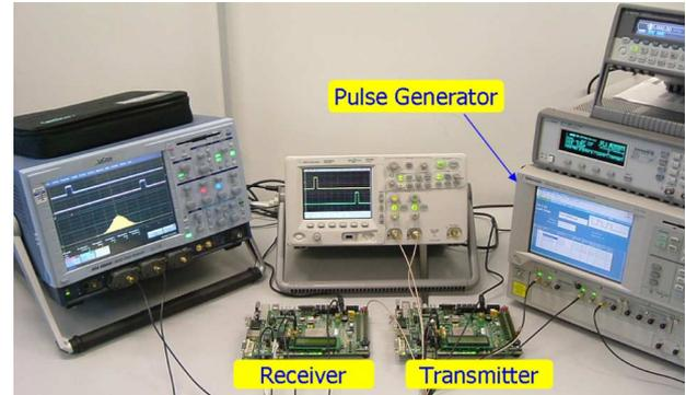
Fig. 9. Experimental setup for latency tests.
