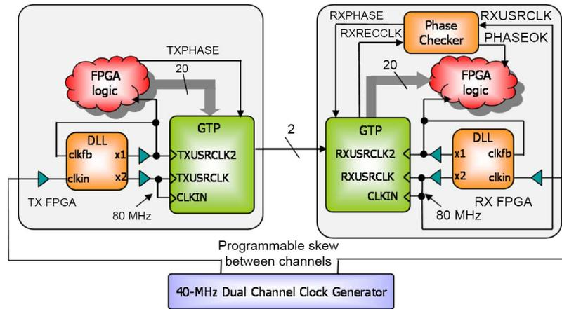
Fig. 7. Adopted clocking scheme for the GTP transmitter and receiver for synchronous operation.
