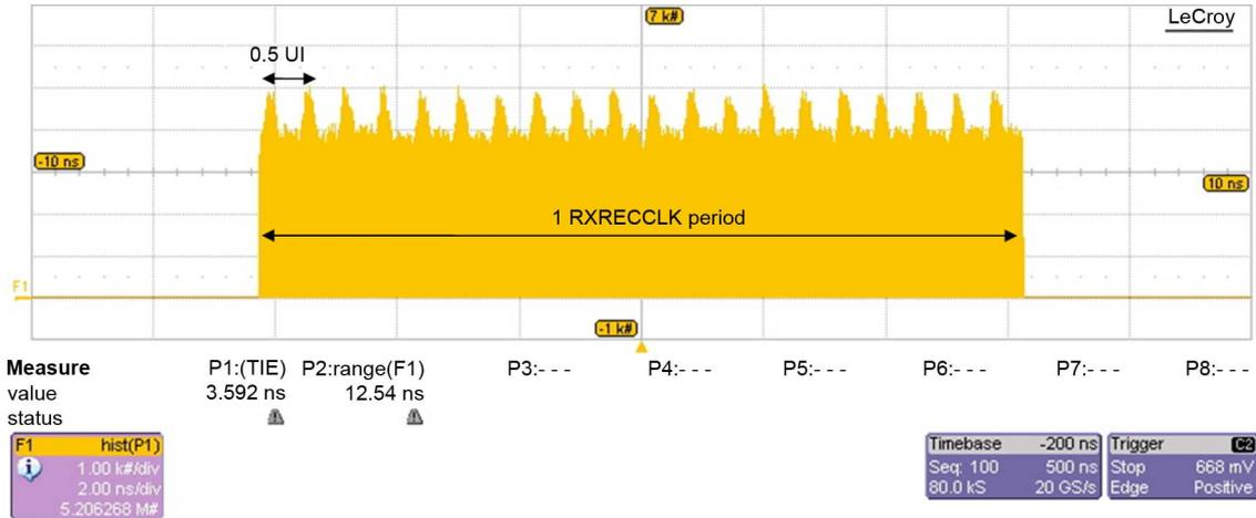
Fig. 8. Histogram showing the relative phase between RXRECCLK and the reference clock when  $\Delta\phi$  does not satisfy the requirements of the phase align circuit.
