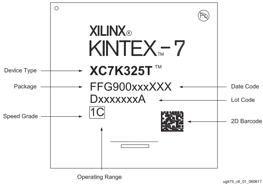
Figure 6-3: Kintex-7 Device Package Marking
