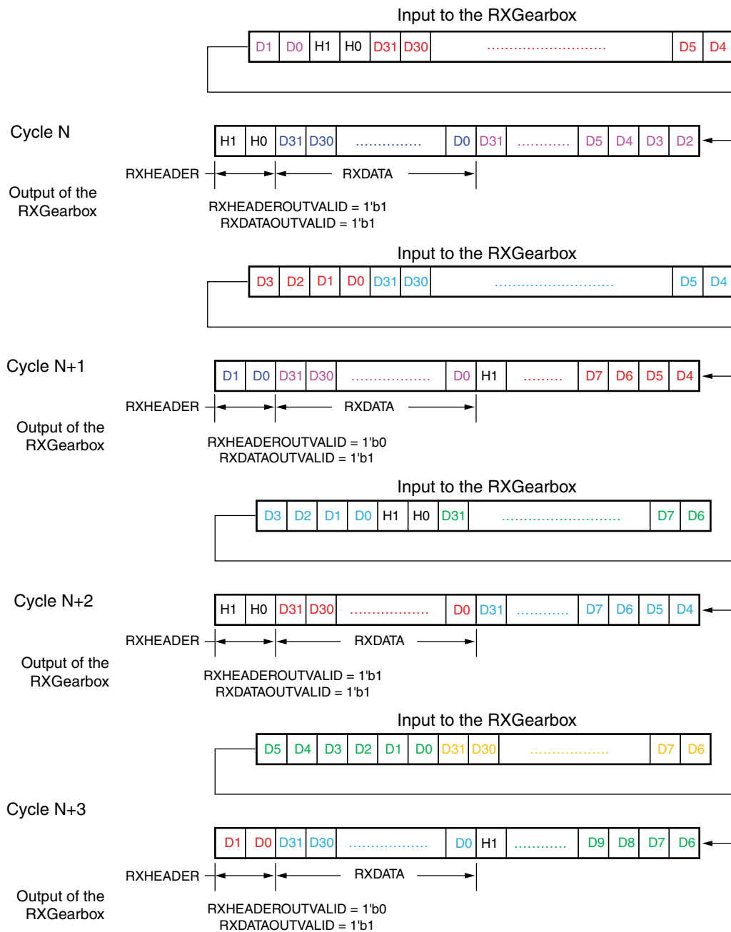
Figure 4-60: RX Gearbox Operation in Normal Mode (GEARBOX_MODE[2] = 1'b0)
